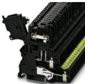
Ground modular terminal block with fuse holder for G fuse insert, cross section: 0.14 - 4 mm 2 , AWG: 26 - 10, width: 6.2 mm, color: black
