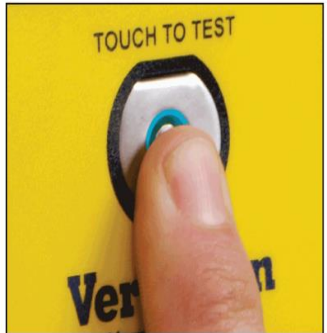
Figure 10. Bridging the test switch's contacts to initiate the test
