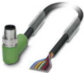
Sensor/Actuator cable, 12-position, PVC, Black RAL 9005, Plug angled M12 SPEEDCON, A-coded, on free cable end, Cable length: 1.5 m
