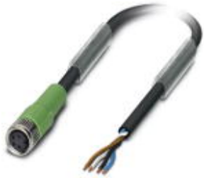
Sensor/Actuator cable, 4-position, PUR, Black RAL 9005, free cable end, on Socket straight M8, Cable length: 20 m
