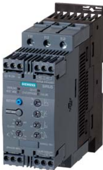
SIRIUS SOFT STARTER, S2, 72A, 37KW/400V, 40 DEGR., AC 200-480V, AC/DC 110-230V, SCREW TERMINALS
