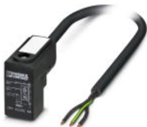
Sensor/Actuator cable, 3-position, PVC, Black RAL 9005, free cable end, on Valve connector CI (9.4 mm), with 1 LED, connected with Z diode, Cable length: 10 m
