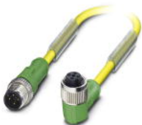
Sensor/Actuator cable, 4-position, PUR/PVC, Yellow RAL 1021, Plug straight M12, A-coded, on Socket angled M12, A-coded, Cable length: 0.6 m, DESINA
