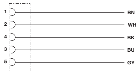
Contact assignment of the M12 socket
