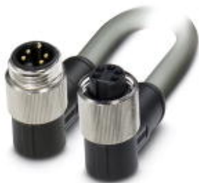
Power cable, 5-position, PUR, Gray RAL 7001, Plug angled 7/8"-16UNF, on Socket angled 7/8"-16UNF, Cable length: 2 m, 2.5 mm 2 conductor cross section, For power supply
