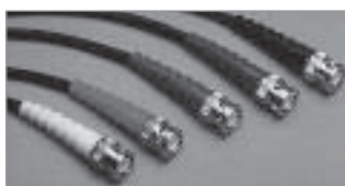
RG-58 Thin Ethernet BNC to BNC Cables Constructed of 50 Ohm, 95% Braid & 100% Foil Shield Cable, 20 AWG Stranded (Belden 9907 Equivalent), Black PVC Cable.
