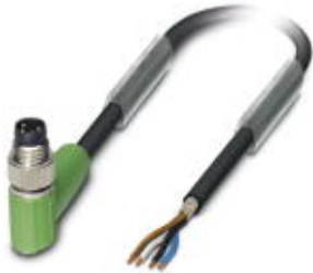
Sensor/Actuator cable, 4-position, PUR halogen-free, black-gray RAL 7021, shielded, Plug angled M8, on free cable end, Cable length: 10 m
