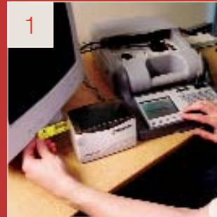
1 On completion of the test routine, choose the type of label you would like. It is then printed automatically from the tester.
