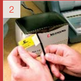
2 Use the peelstick, if needed, to help remove the backing from the panel.
