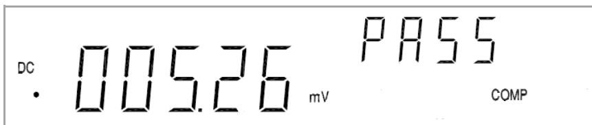
Figure 2-14 Typical Comp operation display
