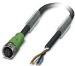
Sensor/Actuator cable, 4-position, PUR, black-gray RAL 7021, free cable end, on Socket straight M12, A-coded, Cable length: 2 m
