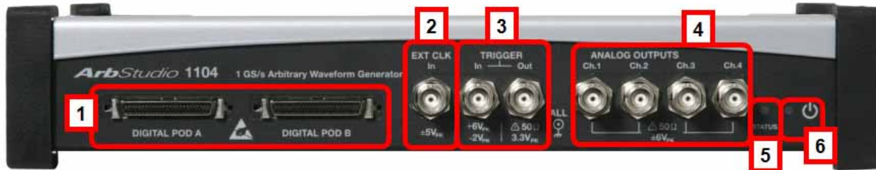
Figure 3-1. This is an image of the ArbStudio 1104 model and therefore has a POD B connector and two additional Channel Outputs. Although digital pods appear on all models, they are only active on 1102D and 1104D models.
