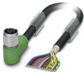
Sensor/Actuator cable, 17-position, PUR/PVC, Black RAL 9005, shielded, free cable end, on Socket angled M12 SPEEDCON, A-coded, Cable length: 3 m
