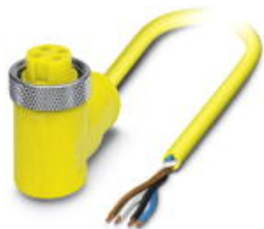
Sensor/Actuator cable, 4-position, PVC, Yellow RAL 1021, free cable end, on Socket angled 7/8"-16UNF, A-coded, Cable length: 6 m
