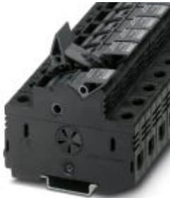
Fuse terminal block, for cartridge fuse insert 10.3 x 38 mm, cross section: 1.5 - 25 mm 2 , AWG: 16 - 4, width: 18 mm, color: Black
