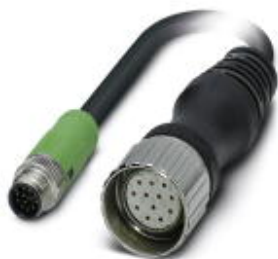
Sensor/Actuator cable, 12-position, PUR/PVC, Black RAL 9005, shielded, Plug straight M12 SPEEDCON, A-coded, on Socket straight M23, Cable length: 5 m
