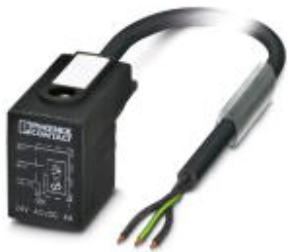
Sensor/Actuator cable, 3-position, PUR halogen-free, black-gray RAL 7021, free cable end, on Valve connector BI (11 mm), with 1 LED, connected with Varistor, Cable length: 5 m
