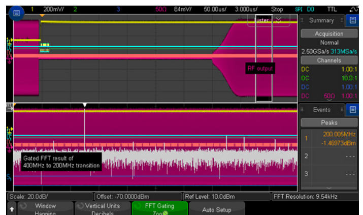
Figure 21d: RF signal settled down at 200 MHz as indicated in the search list.
