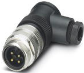
Connector, 4-position, Plug angled 7/8"-16UNF, Screw connection, Knurl material: Zinc die-cast, nickel-plated, Cable gland Pg9, External cable diameter 6 mm ... 8 mm, Contact 4 leading
