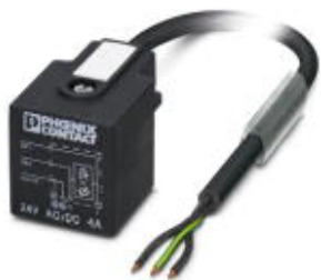
Sensor/Actuator cable, 3-position, PUR halogen-free, black-gray RAL 7021, free cable end, on Valve connector A, with 1 LED, connected with Varistor, Cable length: 5 m
