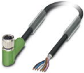
Sensor/Actuator cable, 6-position, PUR halogen-free, black-gray RAL 7021, shielded, free cable end, on Socket angled M8, Cable length: 10 m
