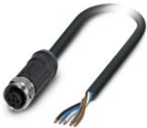
Sensor/Actuator cable, 5-position, PE-X halogen-free, black-gray RAL 7021, free cable end, on Socket straight M12, A-coded, Cable length: 5 m, for outdoor applications, With high-grade steel knurl
