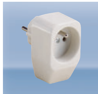
Adapter Thermoplastic fibre glass reinforced contact support, plug side with two earthing systems acc. to CEE 7/VII socket outlet side with earthing system acc. to CEE 7/V
