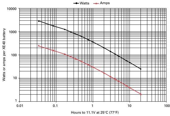
Figure A-16: XE40 discharge data to 11.1V at 25°C (77°F)
