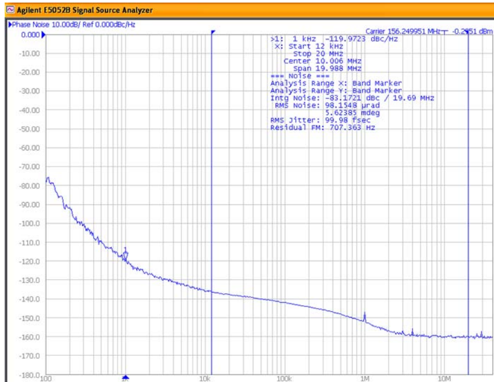
Figure 5. Input = 25 MHz; Output = 156.25 MHz, 2.5 V LVDS
