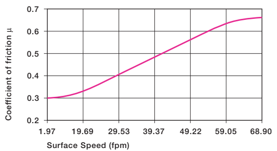
Graph 2.4: Coefficient of friction of iglide® M250 as a result of the surface speed; p = 108 psi
