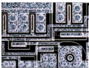
Dark field (DF) observation: Observing only the scattered light by shutting down the direct light to the objectives. The scratches and dust that cannot be viewed in the bright view field can be observed by this method in high-contrast.
