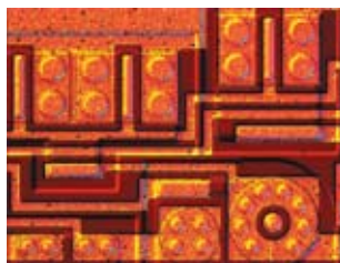
Differential interference contrast (DIC) observation: Effective in detecting fine scratches and steps on the surface of metal, liquid crystal, and semiconductors.
