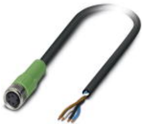
Sensor/Actuator cable, 4-position, PVC, Black RAL 9005, free cable end, on Socket straight M8, Cable length: 5 m
