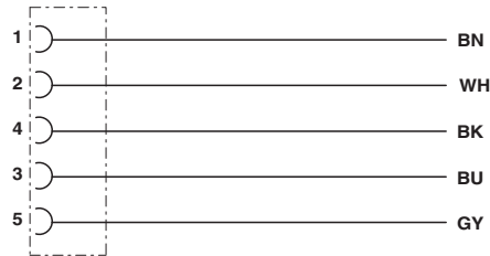
Contact assignment of the M12 socket
