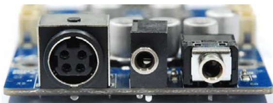
24V Ac/DC adaptor Type (connect with J3 barrel jack)
