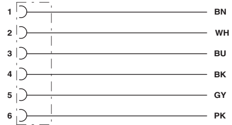
Contact assignment of M8 socket
