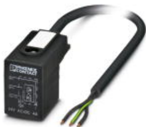
Sensor/Actuator cable, 3-position, PVC, Black RAL 9005, free cable end, on Valve connector B (10 mm), with 1 LED, connected with Z diode, Cable length: 5 m
