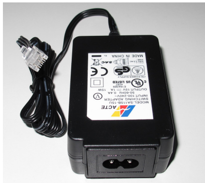
In-line power supply showing 'figure-8' connector at base of image.
