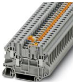
Knife disconnect terminal block, Connection method: Screw connection, Cross section: 0.14 mm 2 - 6 mm 2 , AWG: 26 - 10, Width: 6.2 mm, Color: gray, Mounting type: NS 35/7,5, NS 35/15
