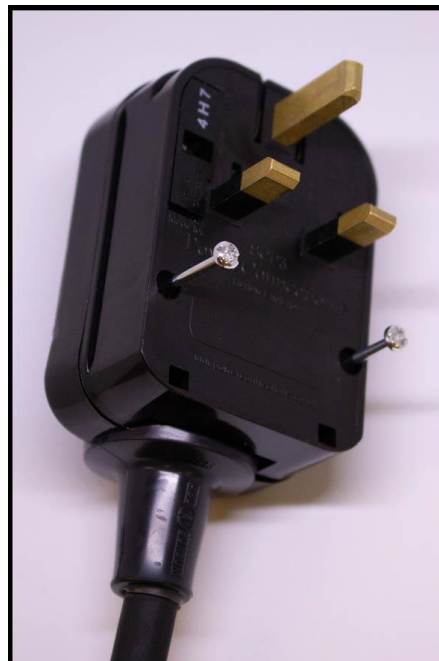
Figure 3 – loosening of screws of converter plug
