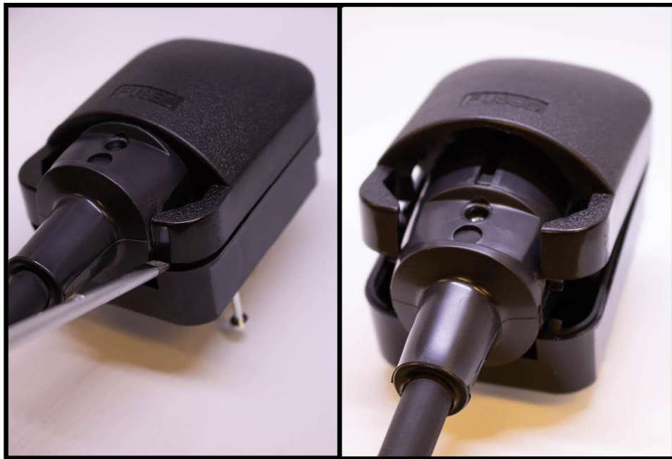
Figure 4 – releasing of the barbed clips or the top housing
