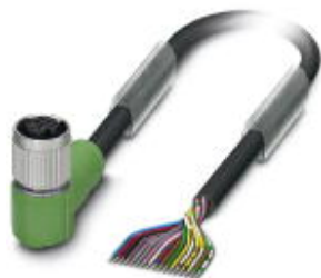
Sensor/Actuator cable, 17-position, PVC, Black RAL 9005, free cable end, on Socket angled M12 SPEEDCON, A-coded, Cable length: 10 m
