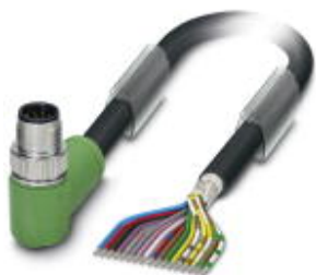
Sensor/Actuator cable, 17-position, PUR/PVC, Black RAL 9005, shielded, Plug angled M12 SPEEDCON, A-coded, on free cable end, Cable length: 10 m
