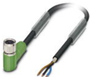
Sensor/Actuator cable, 3-position, PUR halogen-free, black-gray RAL 7021, shielded, free cable end, on Socket angled M8, Cable length: 5 m
