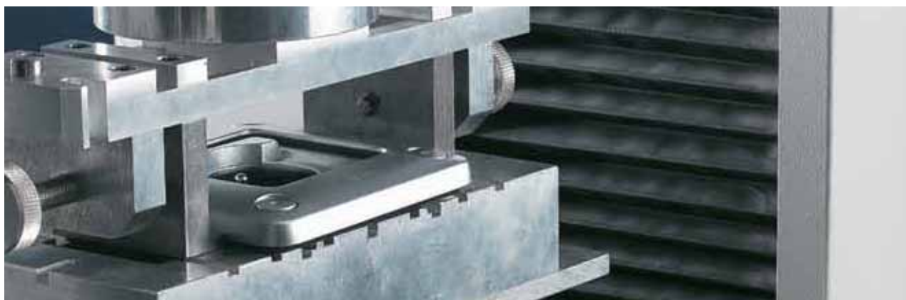
IK 10: MAXIMUM PULL-OFF RESISTANCE | Rounded plate shape to prevent a firm grasp
