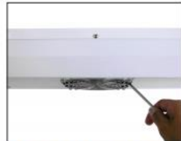
Figure 8. Shorting the ionizer's two fan grills
