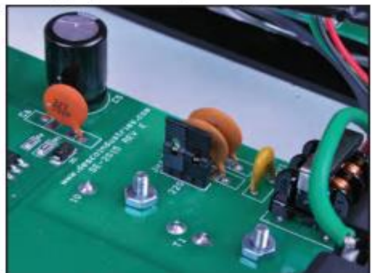
Figure 3. 110 volt jumper setting
