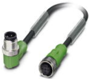
Sensor/Actuator cable, 3-position, PUR halogen-free, black-gray RAL 7021, Plug angled M12, A-coded, on Socket straight M12, A-coded, PIN 2+4 bridged, Cable length: 0.6 m
