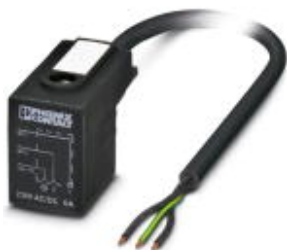
Sensor/Actuator cable, 3-position, PVC, Black RAL 9005, free cable end, on Valve connector BI (11 mm), Cable length: 2 m
