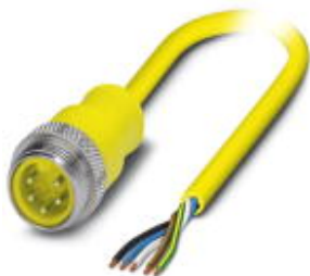
Sensor/Actuator cable, 5-position, PVC, Yellow RAL 1021, Plug straight 7/8"-16UNF, A-coded, on free cable end, Cable length: 2 m
