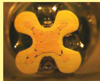
Crimp-cross section HARTING crimp profile
