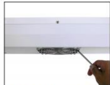
Figure 8. Shorting the ionizer's two fan grills
