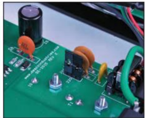
Figure 3. 110 volt jumper setting
