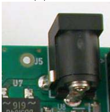
Figure 2-4 . Male JACK Outlet and Wires
