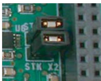
Figure 2-8 . STKX1 and STKX2 jumpers on STK526
