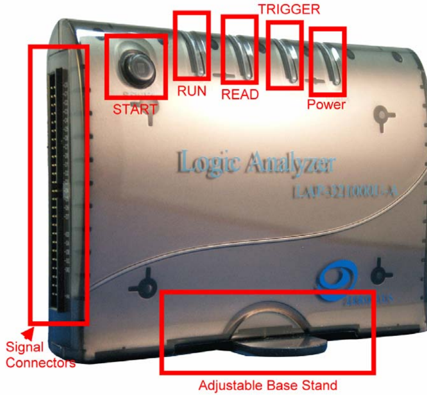
Fig. 1-9: A view of the ZeroPlus Logic Analyzer LAP-A Series. see Fig 1-12 for detailed information on the Signal Connectors .
